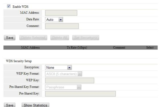
Enable WDS: by default, you can't select the checkbox to enable WDS.
