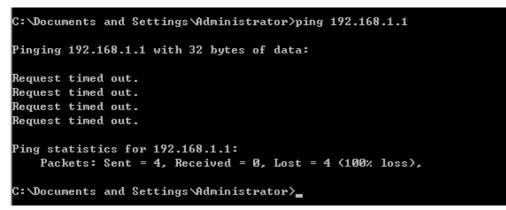
If the result displayed is similar to that shown in the above figure, it means that your PC has not connected to the Router successfully. Please check it following below steps:
